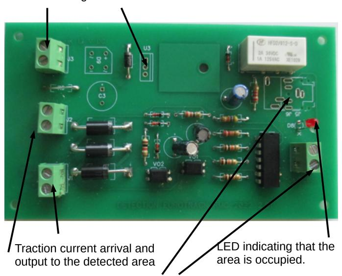
Contact indicating occupancy: terminal block or mono jack socket, for sending to the "Eurotrack block" (contact if the zone is not occupied)
